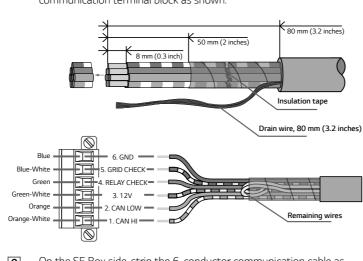
On the SE Box side, strip the 6-conductor communication cable as shown in the figure.
