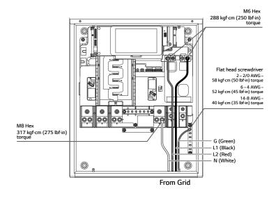
Connect the home load conductors (L1, L2, Neutral, and Ground) to the SE Box backup load terminals
