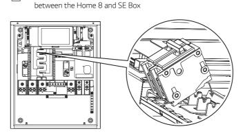
connect the AC conductors to the corresponding terminals
