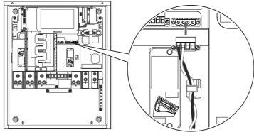
Arrange the power cables and fasten them using a cable tie.
