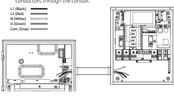
Strip off the AC power conductors (L1, L2, Neutral, and Ground) on both the Home 8 and SE Box sides as shown in the figure below.
