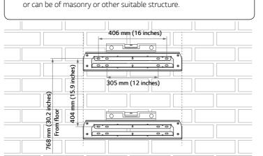
Affix the wall bracket to the wall with screws or anchors. Align the upper and lower brackets so that they are straight
