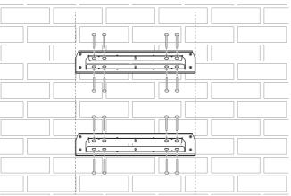
Hang the Home 8 on the wall bracket using the lift.
