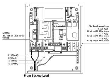
3 Connect the non-backup load conductors (L1, L2, Neutral, and Ground) from the non-backup panel to the SE Box non-backup load
