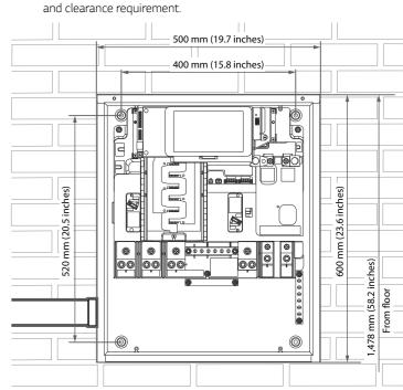
Fix the SE Box with 4EA screws and anchors with O-rings in each Before fastening the screws, place the supplied O-rings on the
